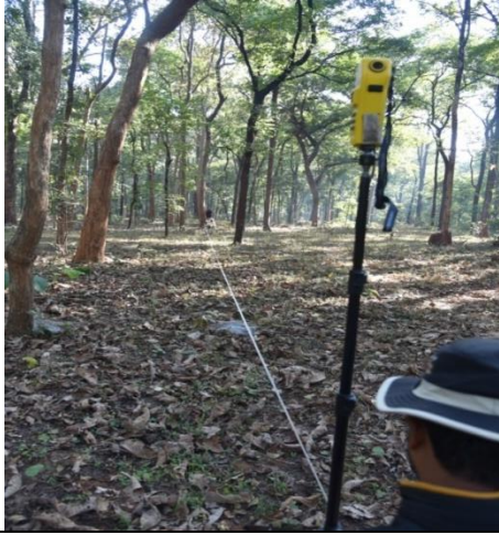
Fig. 14 Measurement of tree diameter at different height segments of Bridelia retusa at Dhamtari forest division using Basal Area Finder (BAF) Scope
