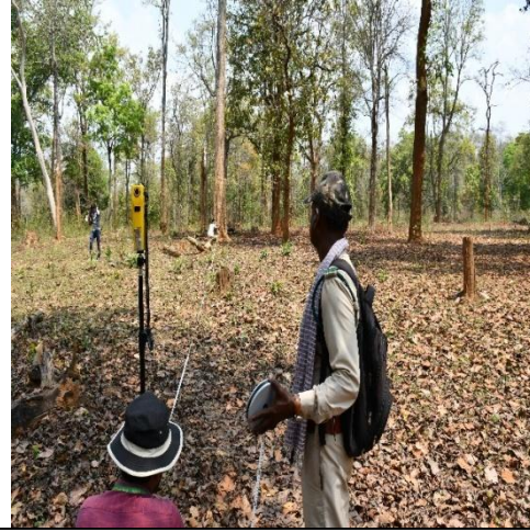
Fig. 15 Measurement of tree diameter at different height segments of Adina cordifolia at Bastar forest division using Basal Area Finder (BAF) Scope
